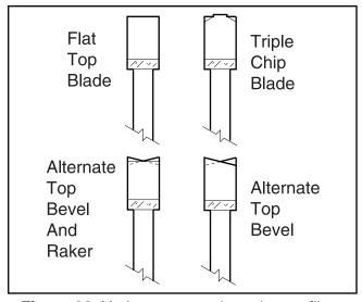
Figure 32. Various saw tooth cutting profiles.
